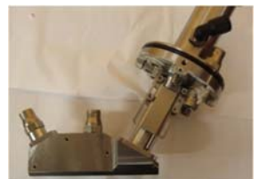
Fig4. New non-emerging cutting head
