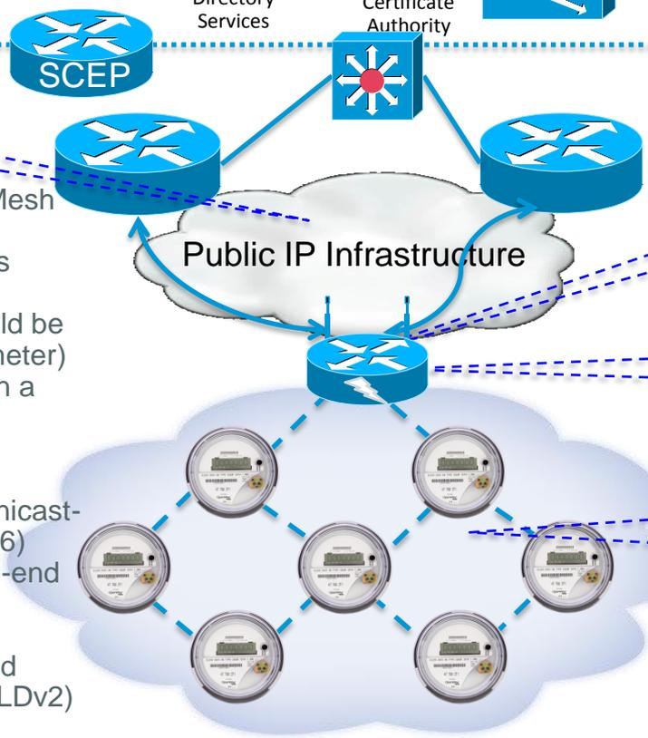
Each Concentrator registers to Multicast group for its specific Mesh domain
