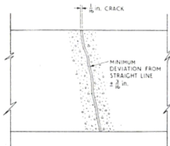
図 1 Typical crack through mass concrete shield
