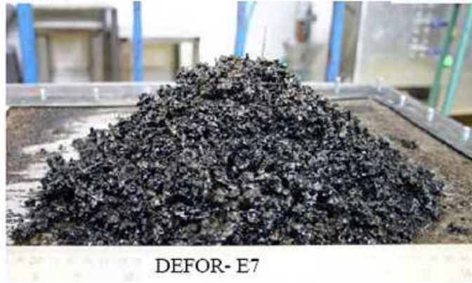
図付 3-6 DEFOR-E 試験後のデブリ状態 [16]
